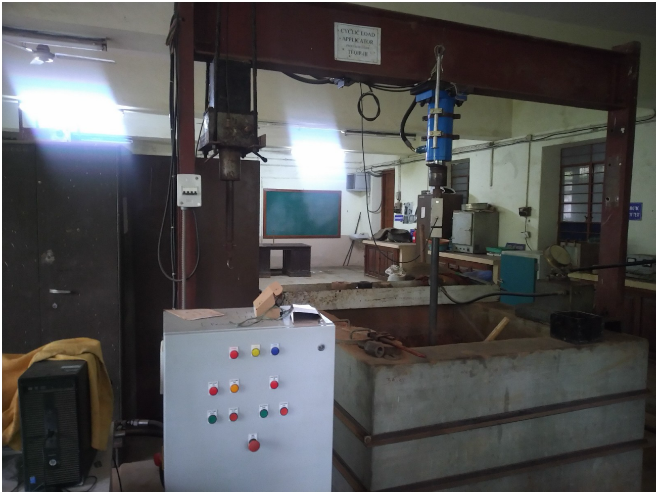
Fig. 7 (b) A view of Plate Load Test Facility after installation of Cyclic Load Applicator
