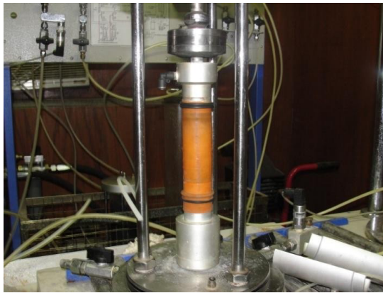
Fig. 2 Specimen before and after the tests in a PC Controlled Cyclic Tri-axial facility
