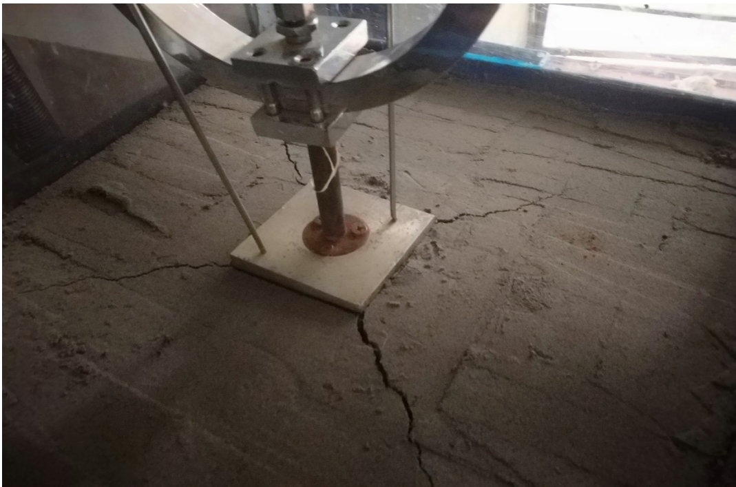
Fig. 18 A view of the test bed after failure
