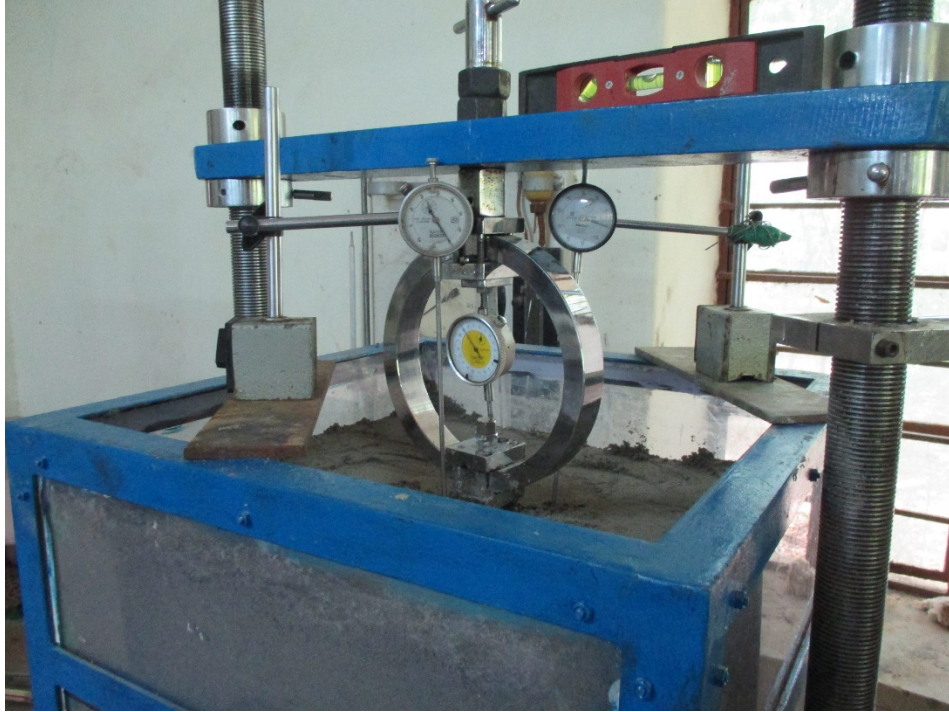
Fig. 17 A view of Test bed with instrumentation placed
