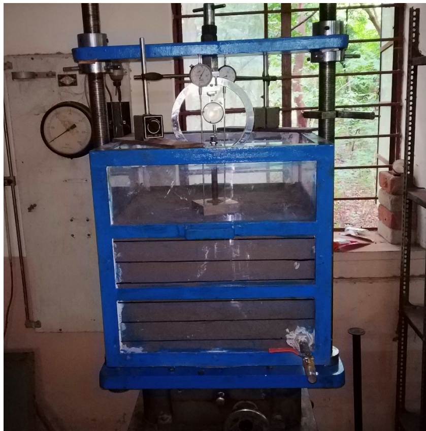
Fig. 16 Modification of an un-used CTM in to Load Test Facility under TEQIP-III
