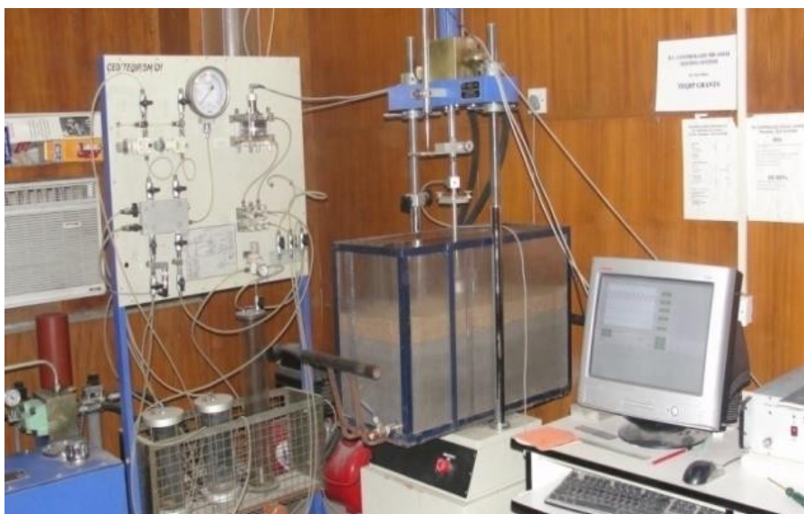
Fig. 1 The PC Controlled Cyclic Triaxial converted in to Cyclic Load Test Facility
